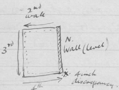
Woods (karapunter) had made five pairs of shutters from the floorboards of the tent that was "lost" in 1947. The trench for the North foundation-wall was finally levelled, shuttering placed in position, concrete mixed and then put in and covered over for the night.
